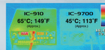
This is a comparison between two transceivers' rear chassis temperatures when continuously transmitting for 15 minutes. The IC-910* rises to 65 °C while the IC-9700 rises only to 45 °C. * Japanese version example when testing at 50 W.
