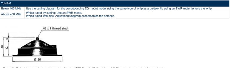
Generally:Order this magnetic base by simply asking for MZG-Mount. (FME-cable and FME-connector are ordered separately).
