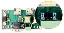
→ Set the jumpers in the audio connection box to **BT-side** which the desktop control unit is connected as shown in the illustration.
